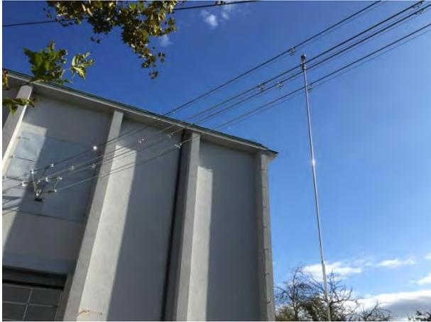
**Figure 7:** A reference testing site for DTR uncertainty evaluation. Two different conductor current loops placed in X configuration to avoid in-between weather disturbance.
